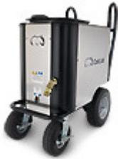
The Cold Jet dry ice blasting uses compressed air to accelerate dry ice pellets frozen carbon dioxide (CO<sub>2</sub>) the high-speed. Compressed air can be supplied in 80 PSI/50 scfm in this process. The dry ice pellets can be manufactured in the plant or purchase. The pellets are made of carbon dioxide suitable for use in food especially FDA approved, EPA and USDA.
